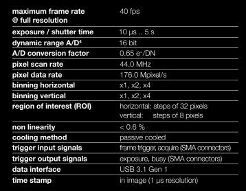
$<sup>^4</sup>$  The high dynamic signal is simultaneously converted at high and low gain by two 12 bit A/D converters and the two 12 bit values are sophistically merged into one 16 bit value.
