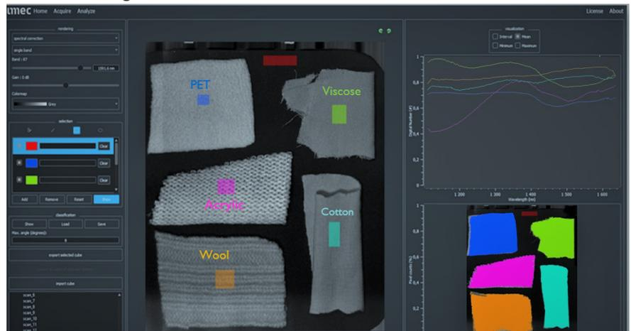
Hyperspectral imaging in the SWIR makes it possible for users to distinguish different types of textiles based on the material and not only on shape and color.
