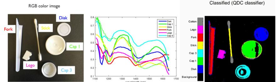
Hyperspectral imaging in SWIR range using imec's snapscan camera with 100 bands enables robust classification of various types of different white color plastics
