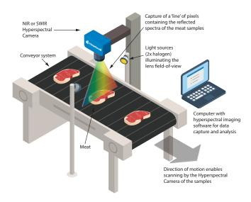
The MV.C NIR can be mounted above industrial conveyor systems or on offline scanning systems for classification-model development or research.
