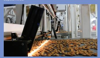
Well-positioned hyperspectral sensors and optimized broadband lighting enable the highest performance in the challenging factory environment.
