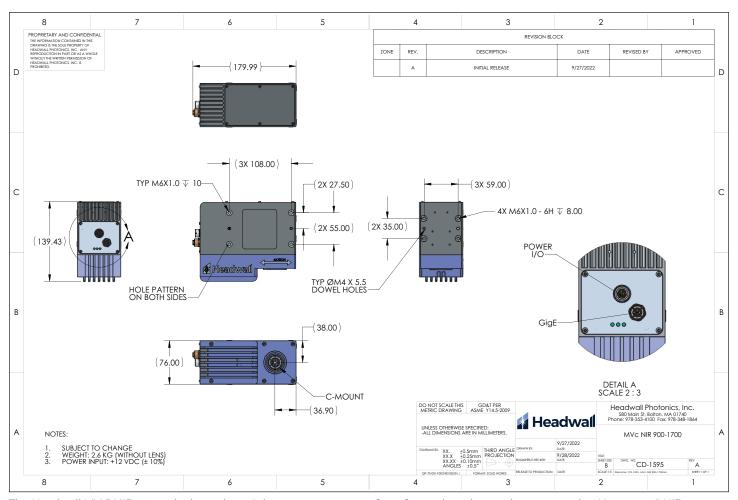
The Headwall MV.C NIR sensor is shown here. It has a more compact form factor than the previous-generation Hyperspec® NIR sensors that it replaces and also features an IP-rated enclosure. All user-accessible ports for power and data I/O are clearly labeled, as is the direction of subject movement. Contact Headwall Customer Support for more complete dimensional drawings if desired.
