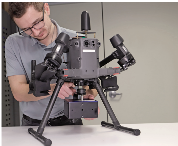
Figure 1. Headwall UAV systems utilize a quick-release mechanism between the drone and the payload that allows easy removal of the sensor suite for transportation or storage.
