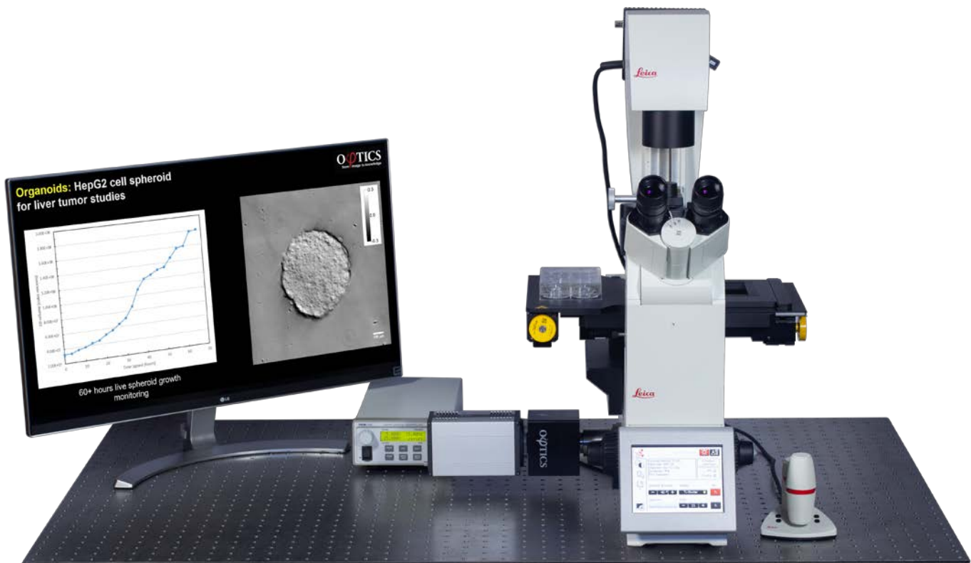
CELLVISTA GLIM PRO module connected to a LEICA DMI8 microscope
